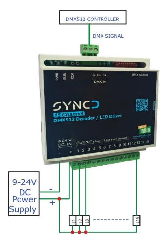
(L1 – L15 is DC load, max 2A per channel)
